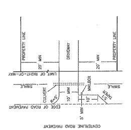
FICE INTENT OF CULVERT IS TO TRANSER AUMOFE IN THE SWALE FROM UPHILL SIDE, TO THE DOWNHILL SIDE, THE INVERTS SHOULD MATCH THE BOTTOM OF THE SWALE WHILE MAINTAINING 12" OF COVER OVER THE PIPE. 12" CULVERT (MIN) 4" BELOW EDGE OF ROAD PAVEMENT -10,-
