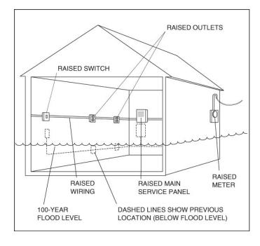
Any electrical system components that are the minimum necessary to meet safety requirements can be below the flood level if energized from a distribution panel located above the flood level and supplied by branch circuits originating from ground-fault circuit-interrupter breakers.
